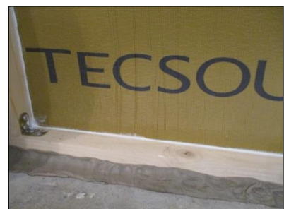
Images 4 to 6 Test element assembly: membrane with wooden frame and perimeter sealing
