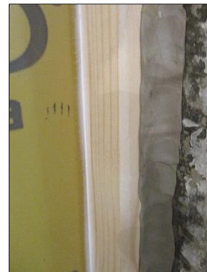
Images 4 to 6 Test element assembly: membrane with wooden frame and perimeter sealing
