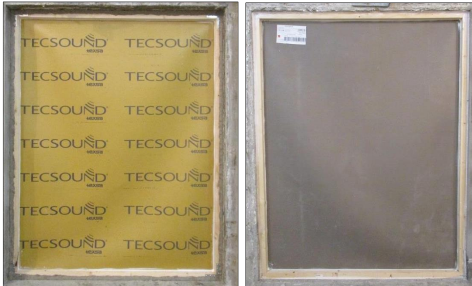
Images 7 and 8 Test element installed into the test opening: view from the source and receiving room
